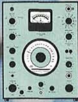
TYPE 1024 SINE OR BAND NOISE 20 Hz TO 20 000 Hz COMPRESSOR
