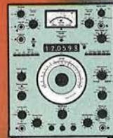
TYPE 2010 2 Hz TO 200 000 Hz 3 Hz TO 1000 Hz BANDWIDTH TRACKING BFO
